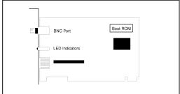
There is one LED on the bracket to indicate the link status.
